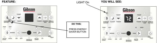
Note: In this mode, the fan will continue to run for 3 minutes after the compressor shuts off. The fan then cycles on for 2 minutes at 10 minute intervals until the room temperature is above the set temperature, at which time the compressor turns back on and cooling stars.
